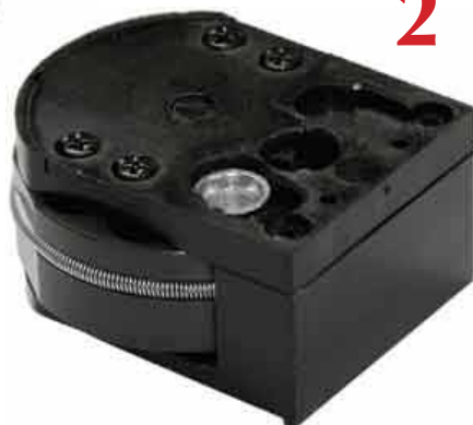
Image 2: Pellet inserted but not properly seated.
